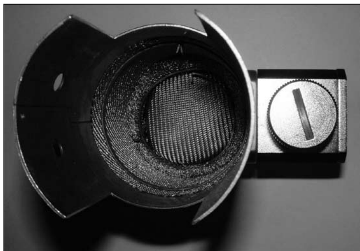
Figure 2. The wick system of an Oxford miniature vaporiser (OMV) consists of metallic mesh
