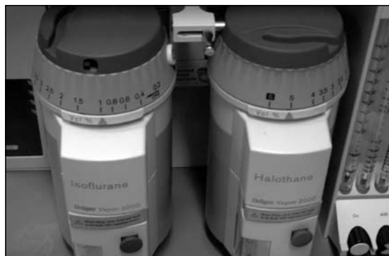
Figure 3. The isoflurane nib is visible and the halothane vaporizer is locked at the 5% position with isoflurane being delivered at 1%
