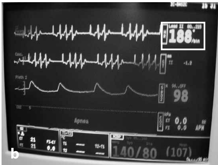
Figure 1. Monitoring screens for a patient who has sinus beats followed by couplets and triplets of pulseless ectopic beats. In (a) the heart rate source (circled) is the pulse oximeter, correctly reading the effective pulse as 40bpm. In (b) the ECG has been selected as the heart rate source, recording a rate of 188 per minute (square), that corresponds to the number of ECG complexes, whether they generate an effective cardiac output or not. Either of these selections can be misleading if the ECG or pulse oximetry monitoring is viewed in isolation.
